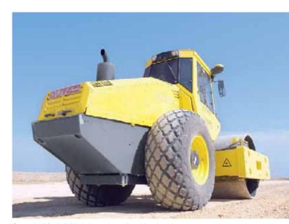
Customised for individual site work: totally enclosed engine compartment.
