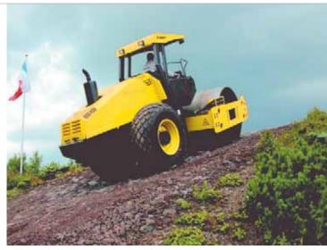
Power on gradients: with no-spin and manual slip control.
