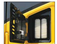
External air conditioner filter
