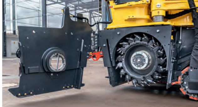
Exchangeable carbide wear protection of the milling box and milling drum.
