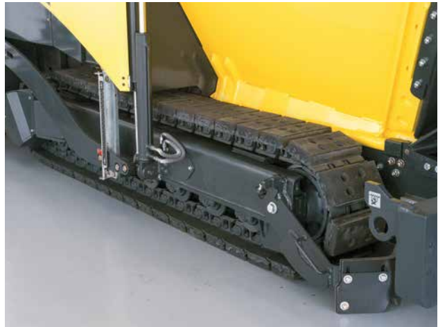
Long crawler tracks ensure dead straight paving.
